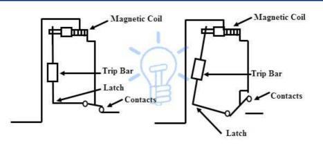
Under short circuit or heavy overload conditions, magnetic tripping arrangement comes into the picture. Under normal working condition, the slug is held in a position by light spring because magnetic field generated by the coil is not sufficient to attract the latch. When a fault current flows, the magnetic field generated by the coil is sufficient to overcome the spring force holding slug in position. And hence slug moves and then actuate the tripping mechanism.
