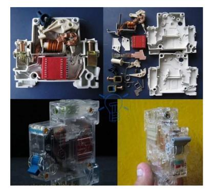
The thermal tripping arrangement consists of a bimetallic strip around which a heater coil is wounded to create heat depending on the flow of current. The heater design can be either direct where current is passed through bimetal strip which effect part of electric circuit or indirect where a coil of current carrying conductor is wound around the bimetallic strip. The deflection of bimetallic strip activates the tripping mechanism in case of certain overload conditions.
